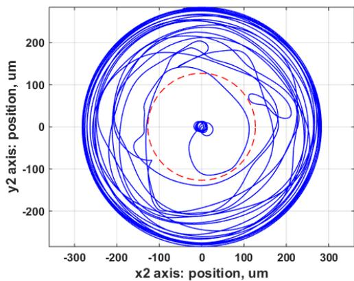
Fig. 10. Simulation 1 position orbit; impulse from sudden unbalance followed by backup bearing whirl w/no IRC.
