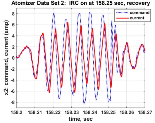
Fig. 8. Current command and coil current vs. time; IRC activates at 158.25 sec.
