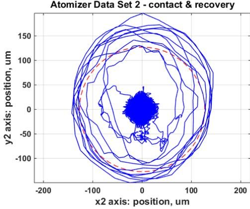
Fig. 7. Orbit at upper radial position sensors during impulse and recovery.
