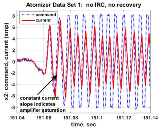
Fig. 6. Current command and coil current vs. time during backup bearing whirl, showing saturation.
